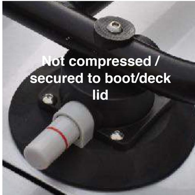
If the cup does not secure to the boot/deck lid you may need to clean the surface or move the rack to a more suitable mounting position.
